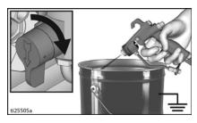
Turn pressure control to Fast Flush. Hold gun against grounded waste pail.
