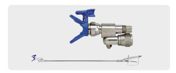
A potential problem when using an extension is paint spitting or dripping from the spray tip. An easy solution is to fit a CleanShot™ valve on the end of the extension.
